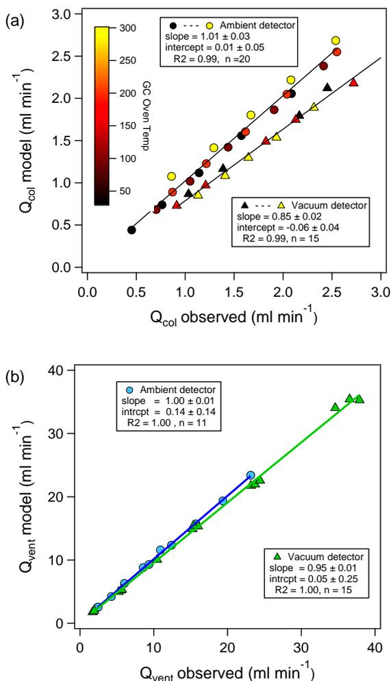
**Figure 4.** Model vs. measurement of average column flow (a) and vent outlet flow (b) for cases of FID (ambient)- or MS (vacuum)-based detection. For the column flow, the oven temperature (color of points) is used to adjust the helium viscosity in the flow model.
