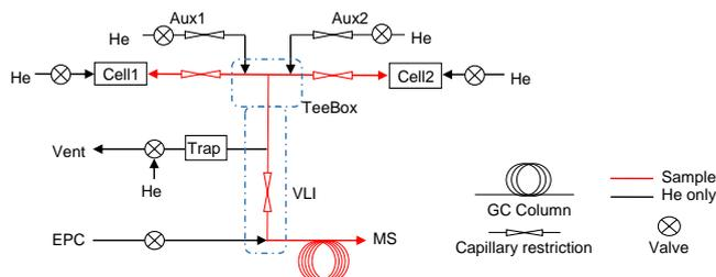
**Figure 3.** Modified valveless injection scheme incorporating two parallel sampling cells to be analyzed sequentially after the samples are initially transferred to a secondary focusing trap. Auxiliary purge valves (Aux1 and Aux2) are used to avoid cross transfer of sample between parallel cells. Dashed squares delineate integrated VLI manifold and a separate heated box for the additional tees (“TeeBox”). Atmospheric sampling lines for both CTD cells are omitted for clarity.
