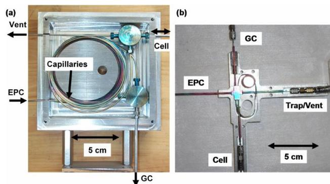
**Figure 2.** (a) Prototype valveless system using discrete components including a pair of zero dead volume tees and two capillary coils. (b) Integrated capillary manifold version of the VLI replaces the discrete tees with a miniature bored manifold into which five capillaries are permanently brazed. The control capillary is seen as a coiled loop connecting one side of each interior tee.
