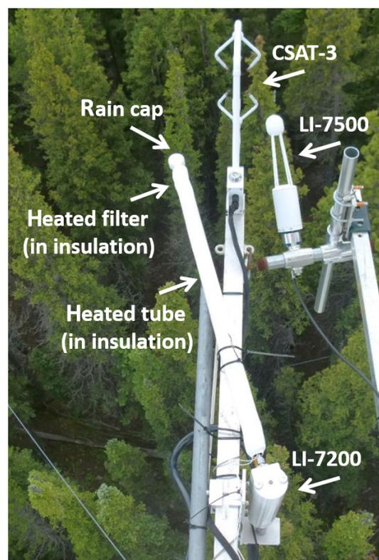
**Figure 2.** Field test setup at the Niwot Ridge US-NR1 Ameri-Flux site. A LI-7200 enclosed-path IRGA and a LI-7500 open-path IRGA are operated side by side next to a CSAT3 sonic anemometer. The LI-7200 gas sampling system consists of rain cap, filter and tube, as well as insulation and adjustable heating of the filter and tube.
