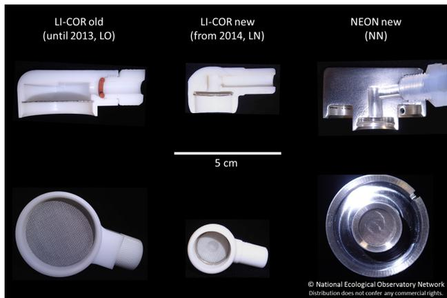
**Figure 1.** Three selected rain cap designs tested in this study. Top row: cross sections of each rain cap showing their internal volumes. Bottom row: rain cap inlets with screens that face downwards in typical field deployments.
